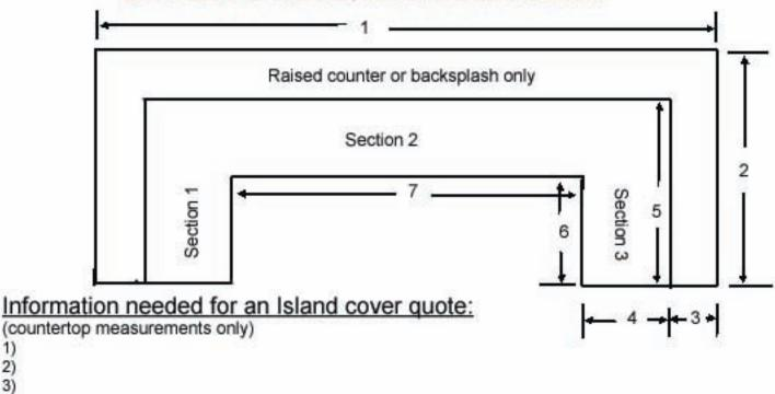
(If other side of U is larger or smaller, then measurements 2 - 6 are needed for that side.)
